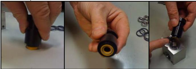
Insert the new seals into the pump body using the SPEC seal insertion tool provided in the kit and press the seal into place. (**Note: the spring side of seal is placed toward the pump body.**)
